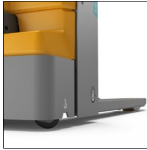
Optimal stability due to spring load support wheels
